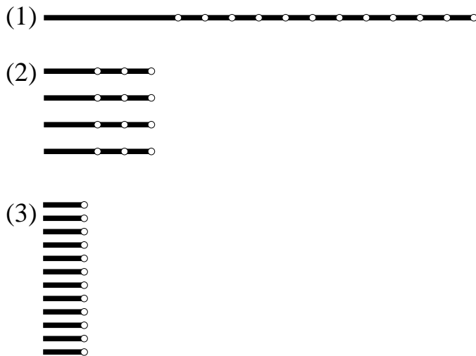
Figure 13. Three possible Markov Chain Monte Carlo strategies for obtaining twelve samples using a fixed amount of computer time. Computer time is represented by horizontal lines; samples by white circles. (1) A single run consisting of one long ‘burn in’ period followed by a sampling period. (2) Four medium-length runs with different initial conditions and a medium-length burn in period. (3) Twelve short runs.
